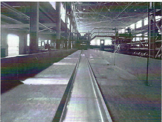
fig. 4 The Massena fabricating mill rolling sections that were each 90 feet in length with an aluminum channel at center of photo. Photo courtesy of NAPHA. 6
